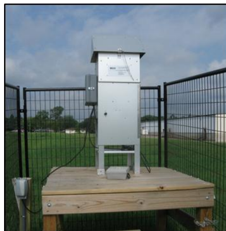
High-volume TSP Sampler
