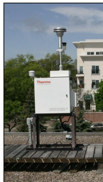
Low-volume PM 2.5 filter monitor
